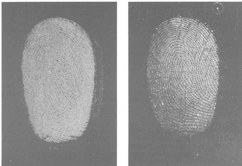
FIG. 3—Identical fingerprints developed with bright magnetic flake powder, (a) where an excess amount of flake powder has been deposited, causing the print to be temporarily obscured, and (b) after the excess flake powder has been removed with a small rare-earth permanent magnet, causing the ridge pattern to be revealed.
